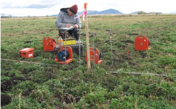
Figure 1 - D.C. Resistivity Crew In Operation
