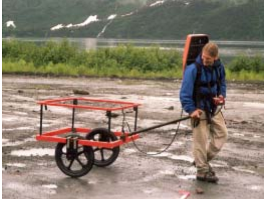
Geonics EM61 "Metal Detector", in Whittier, AK
