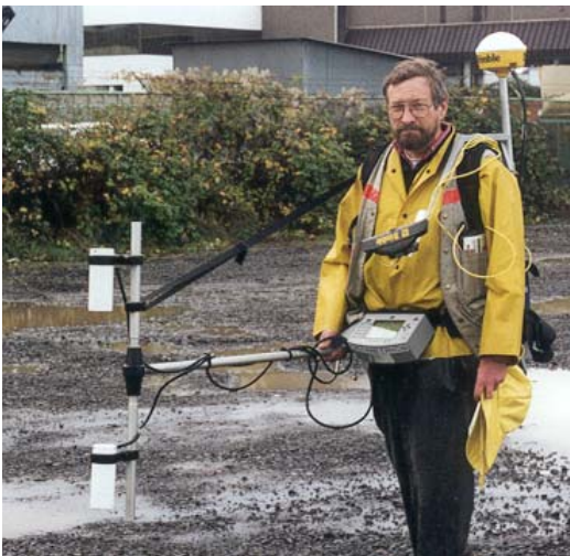
Geometrics G858 Magnetometer/gradiometer with Trimble Ag132 GPS unit, swathing light bar and non-magnetic backpack.
