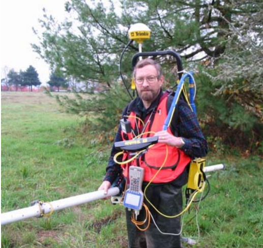
Geonics EM31 Terrain Conductivity Meter with Trimble Ag132 GPS unit, swathing light bar, Allegro field computer, and non-conductive backpack.
