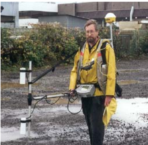
Geometrics G858 Magnetometer/gradiometer with Trimble Ag132 GPS unit, swathing light bar and non-magnetic backpack.
